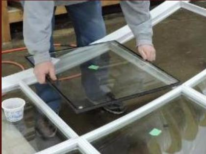
Dry fitting the glass to ensure proper fit
