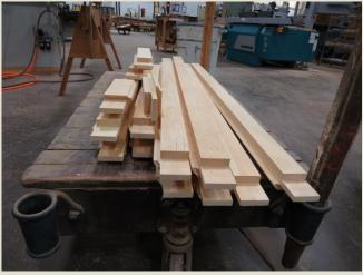
(Left) Baseboard, trim, and door casing pieces ready to be delivered and separated for ease in locating the correct pieces; (Right) Knock down door frames with stops.
