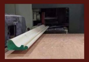
The door casing and trim was fabricated from Poplar. Custom knives were used to match the profile from the specifications provided by the customer. The equipment used to create the casing and trim was a 5-head moulder.
