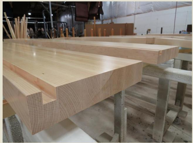
Each of the stair treads are comprised of seven equally sized edge-glued pieces of maple that are 48" wide.
