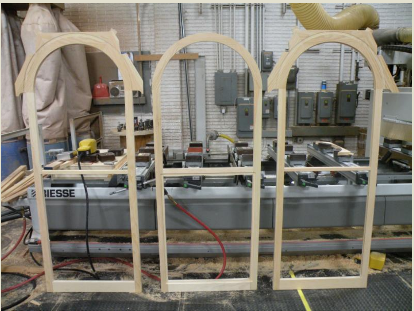
Here is a photo showing the before and after of the half-round curve being cut on the CNC.
