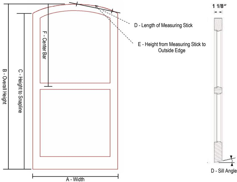
**Note:** Center bar is measured from the top of the storm window to the middle of the center bar.
