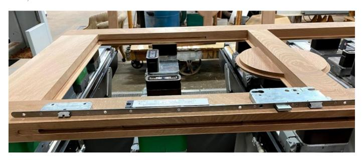
Our CNC is individually programmed to accurately route out for the hardware. The locking system is then installed and hidden seamlessly in the door stile. The points of contact are allowed clear access and with the turn of one button, all three locks are engaged. It is available for use with a variety of handlesets that appeal to all styles.
