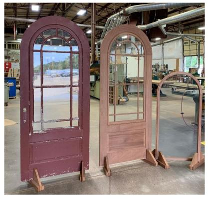
This was a unique storm and screen door that our customer wanted to match. The existing storm door contained an insert with prairie-style lites that highlighted the arched top of the door. The customer wanted to maintain the look with a new door.
