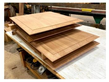
More of the gorgeous Mahogany grain pattern is visible on the solid wood panels for the interior of the door. The profile of the interior panel matches the exterior panel and the wood stop that holds them in place is exactly the same profile used on the exterior.
