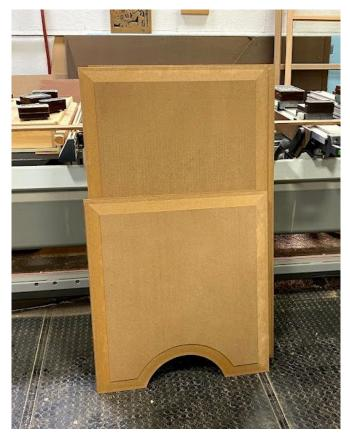
The exterior panels are fabricated of a weather-resistant material that works well with painted doors. The panel raise shows very clean lines which is set off by the round of the lockrail for the doorknob.
