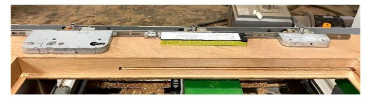
We also have the ability with our CNC to route for wiring within the door. This lets you have a custom wood door with modern security features. Whether you prefer glass options or solid panels to fit your style, we work with our customers to ensure the design works for both style and hardware.
