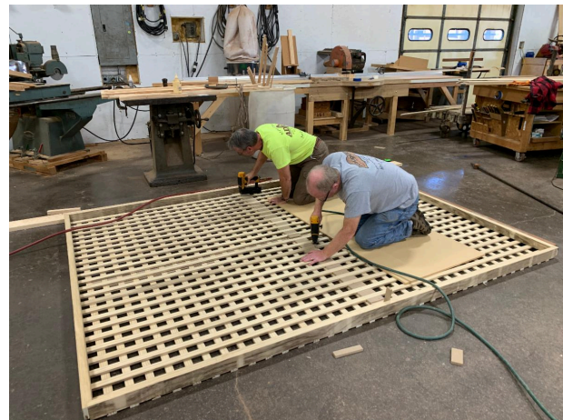
Securing all of the trellis pieces together.
