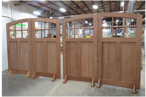
Flat panels added; ready for finishing
