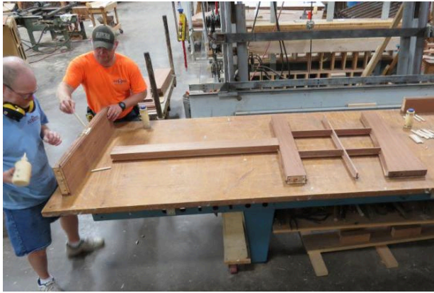
Glue up of door
