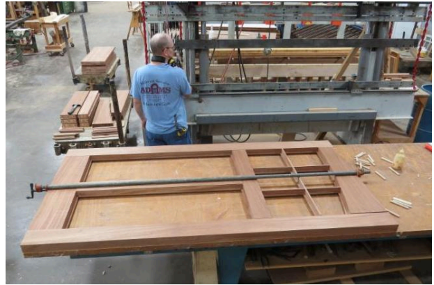
Preparing to clamp
