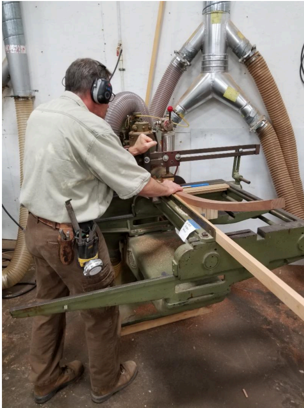
Tenoning the Rails
