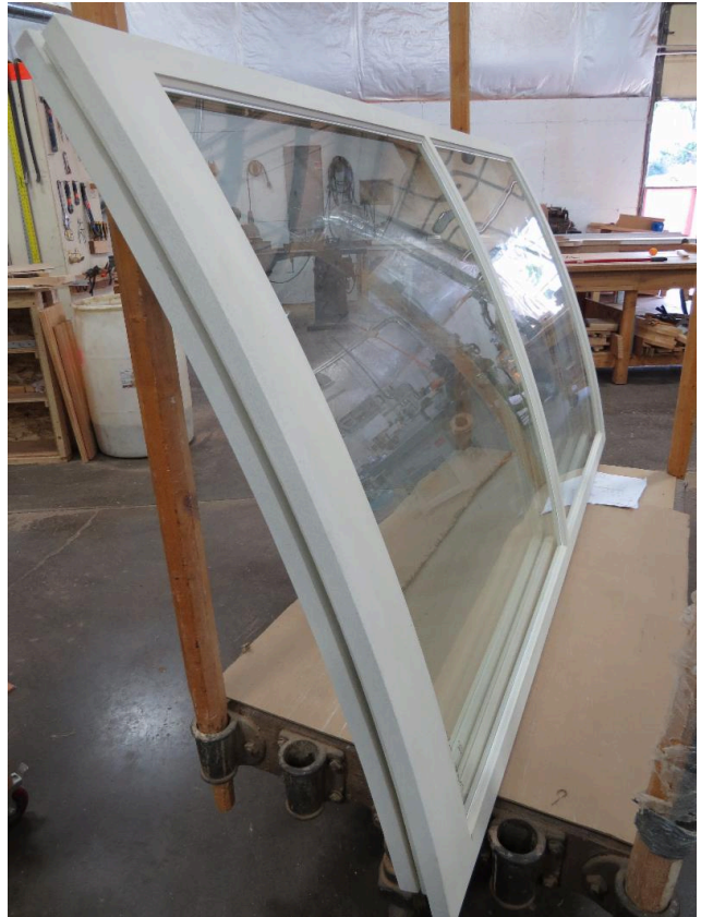
Completed Storm Window
